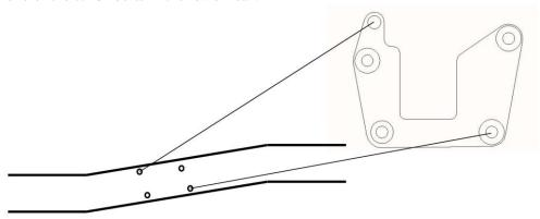
• With the bracket attached to the frame with the aforementioned holes and using it as a template, use a 7/16" drill bit to drill two new required holes as shown below.
