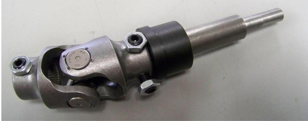
2) Mock up your column to your steering box and determine the length of the complete column including the new U joint. Mark the top of that U joint where it will mate to your  $\frac{3}{4}$ " steering shaft. Cut that  $\frac{3}{4}$ " shaft  $\frac{3}{4}$ " longer to provide  $\frac{3}{4}$ " engagement of that joint. Then mark the mast jacket 1" shorter than the  $\frac{3}{4}$ " shaft and cut it off square. Deburr the inside of the mast jacket and check the fit of the new plastic lower bushing.
