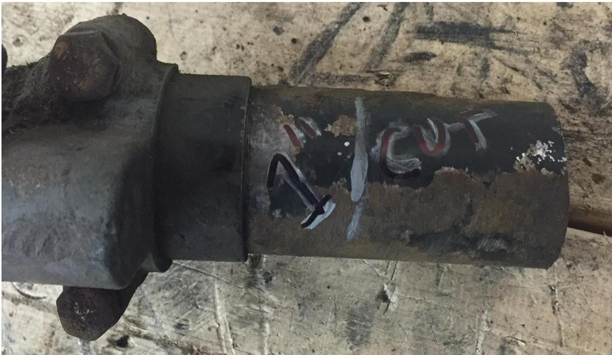
3) Next set the  $\frac{3}{4}$ " shaft from the kit next to your  $\frac{3}{4}$ " main steering shaft. As shown below, mark that original shaft  $3 \frac{5}{8}$ " above the trimmed shaft for cutoff. The turned down end of the new shaft end will be inserted into the old shaft with a  $\frac{1}{8}$ " gap for welding. The overall length should match the length calculated earlier before this cut off.
