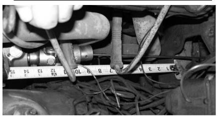
2) Transfer above measurement onto steering column.
